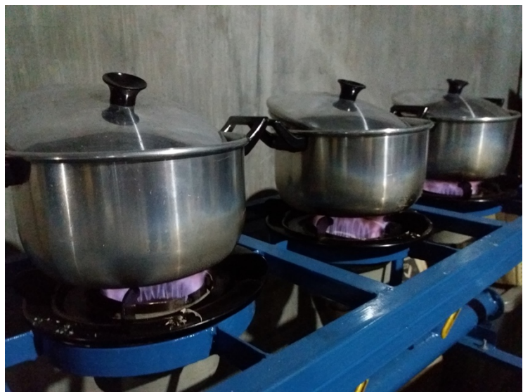
Figure 2. Pictorial of the Three Burners with Flame during Operation.
